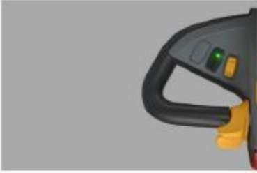
Four colored LED battery meter
