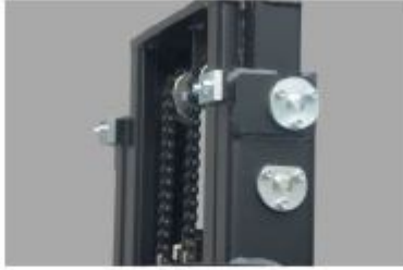
Reinforcing ribs are set between the inner and outer masts
